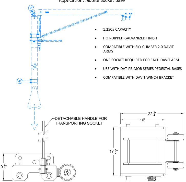
DAVIT IS CAPABLE OF SUPPORTING 5,000 LB. ULTIMATE LOAD AND 1,250 LB. ALLOWABLE LOAD. DAVIT MAY FAIL DUE TO IMPROPER INSTALLATION OR INADEQUATE SUPPORTING STRUCTURE. SERIOUS INJURY OR DEATH MAY RESULT FROM DAVIT FAILURE. INSTALLATION OF DAVIT MUST BE PERFORMED UNDER THE SUPERVISION OF A PROFESSIONAL ENGINEER WITH EXPERIENCE IN SUSPENDED ACCESS EQUIPMENT. ADDITIONALLY, DAVIT SHALL BE TESTED UNDER THE SUPERVISION OF A P.E. AND CERTIFIED BEFORE PLACING INTO SERVICE.
